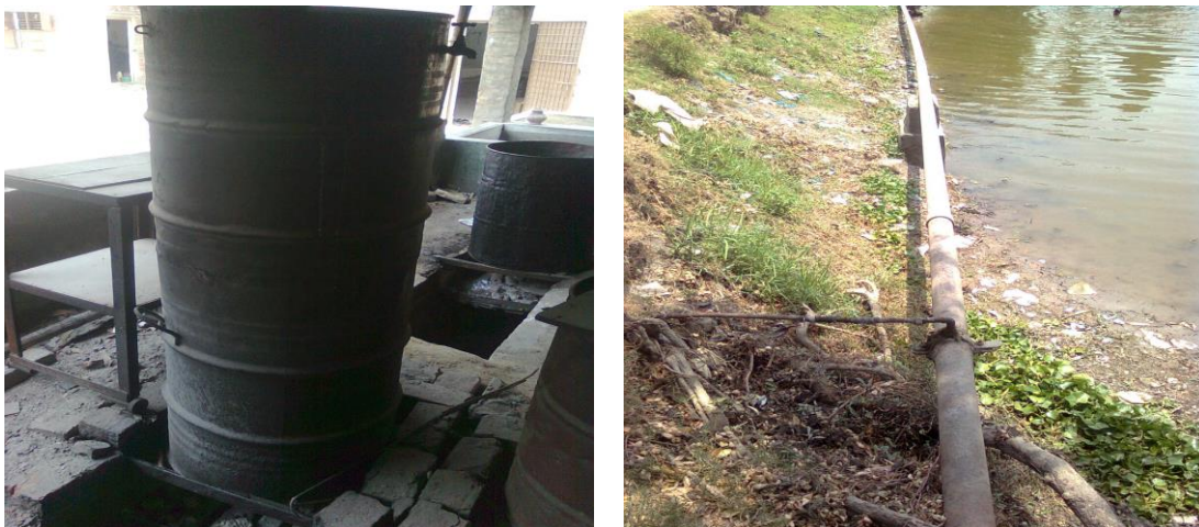
Fig. 3: Washing drum and pipe line for dumping at pond
