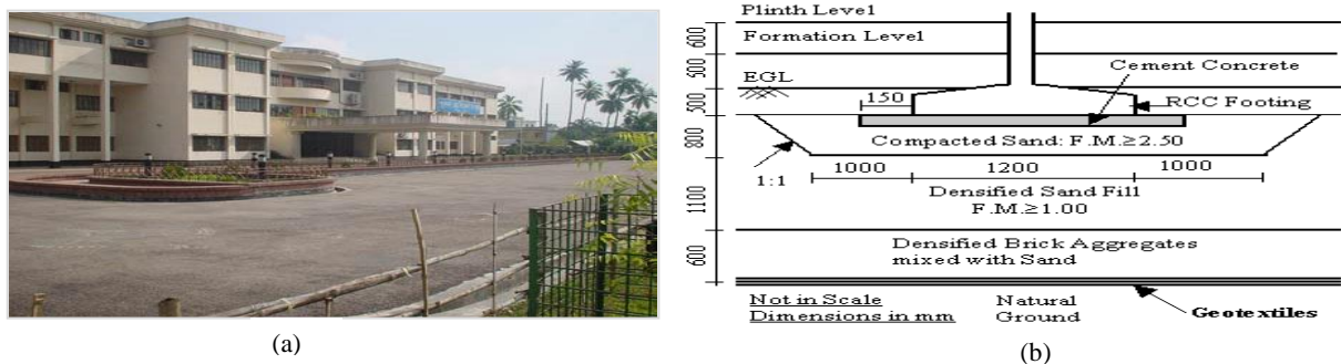
Fig. 2. (a) Academic building of Khulna Medical College and (b) foundation system (Alamgir and Chowdhury, 2004)
