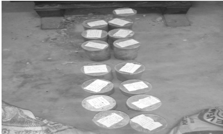
Fig. 1(c): Cylinders prepared for compressive strength test
