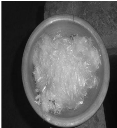
Fig. 1: Recron-3S polymer modified fibre.
