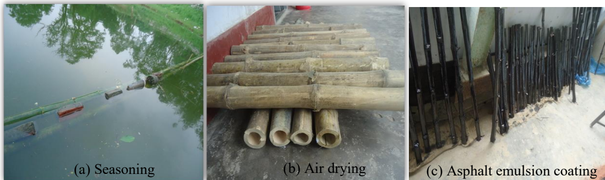
Fig. 2: Preparation of bamboo sticks (a) Seasoning (b) Air drying (c) Asphalt emulsion coating
