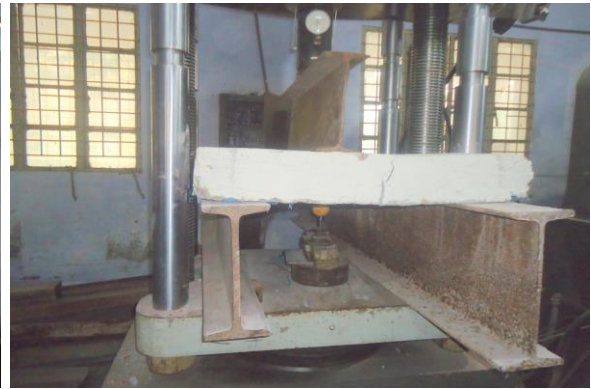
Fig. 6: Flexural test of slab
