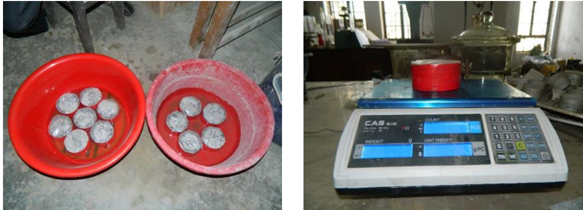
Fig. 6: Experimental setup of water sorptivity test
