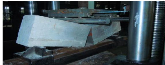
Fig. 4: Failure of crack beam by using brick chips
