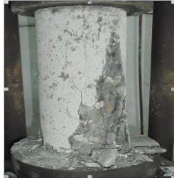
Fig. 1 : Cylinder Compressive Strength Test
