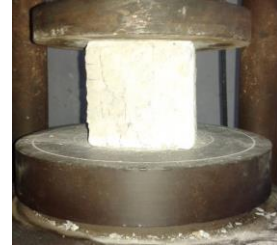
Fig. 2 : Specimen Under Applied Compression Force
