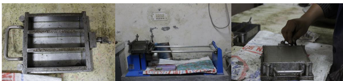
(a) Mould for compressive strength test (b) Jolting apparatus for compaction (c) BDS EN mortar filled moulds
