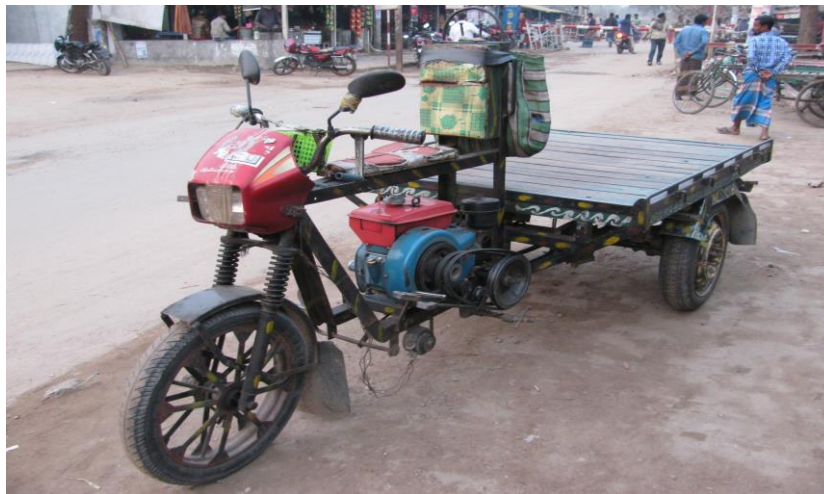
Fig. 1: Motorized rickshaw flatbed with 3 HP Chinese engine
