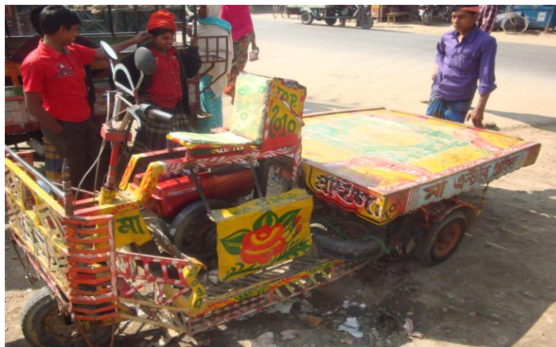
Fig. 2: Motorized flatbed heavy rickshaw or 'vangari'
