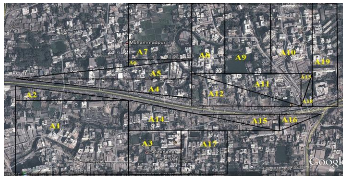
Fig. 3: Various Catchment Areas for determining the actual discharge in Mirza khal
