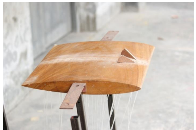
Fig.5: Constructed airfoil with vortex generator
