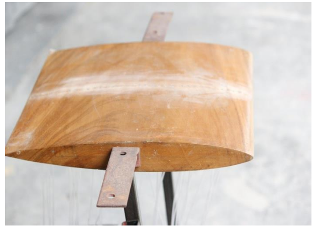
Fig 4: Constructed airfoil of NACA 0012
