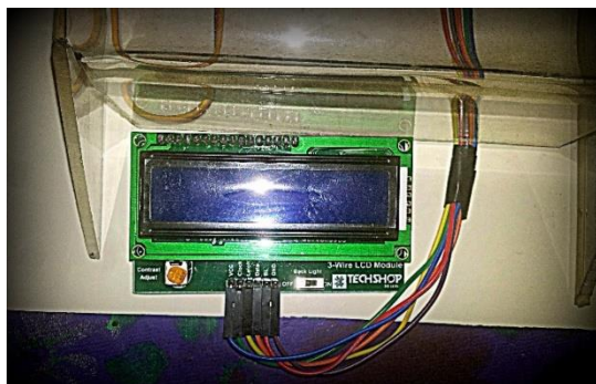
Fig.10: 3-wire LCD Connections
