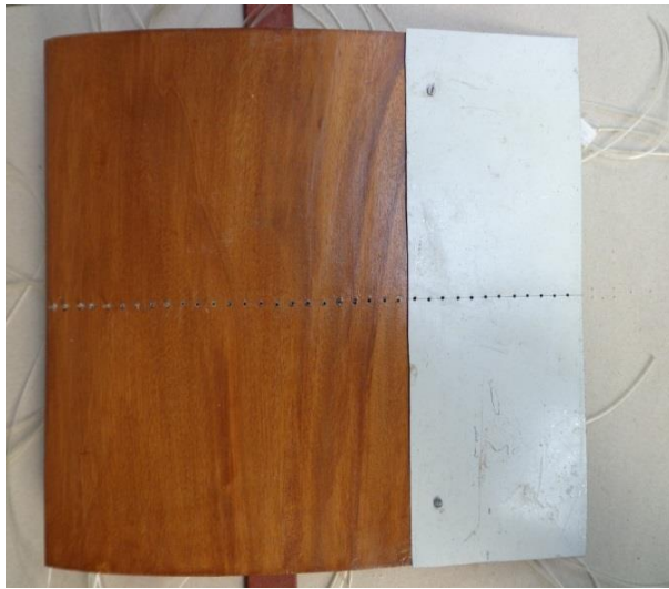
Fig.2: NACA0012 airfoil model attached with a Galvanized Iron (GI) static extended trailing edge.
