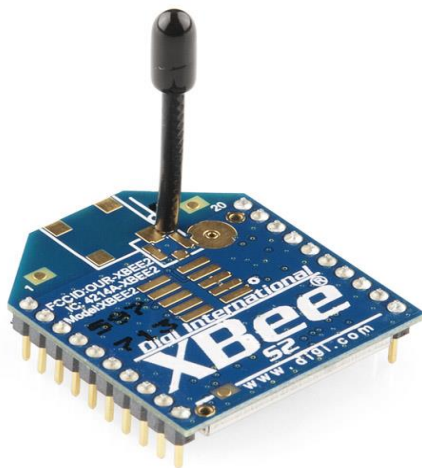
Fig.2: Zigbee 2mW wire antenna series 2 module
