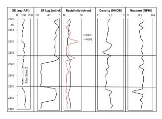
Fig.2: Composite log responses of the hydrocarbon bearing Zone 2 (2337-2350 m) identified in Mio-Pliocene sandstones of the well Rashidpur-4, Bangladesh [25].
