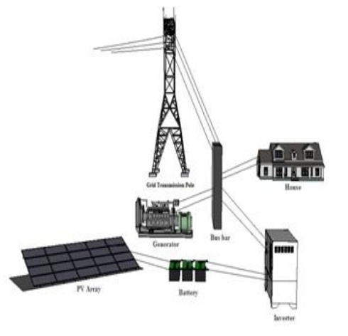
Fig.2: Single line diagram of hybrid energy system [permitted from Ref.21]
