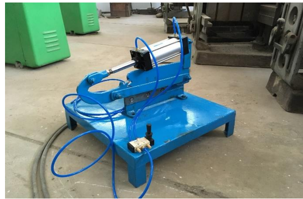
Fig 8: Real view of Pneumatic sheet metal cutting machine.
