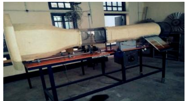
Fig. 08: Wind tunnel setup [6]
