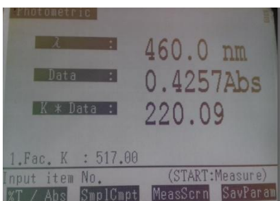
Fig. 9: Absorbance of methyl Orange solution where activated carbon was soaked which is activated by 25% Calcium Chloride Solution
