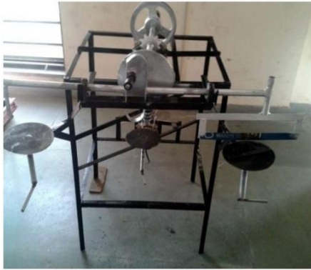
Fig 2.1: Pedal powered Multipurpose Machine
