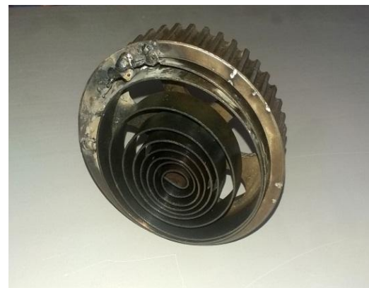
Fig. 4: Flat spiral spring enclosed in gear.
