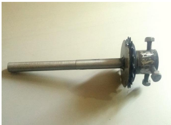
Fig. 6: Alteration of freewheel attachment
