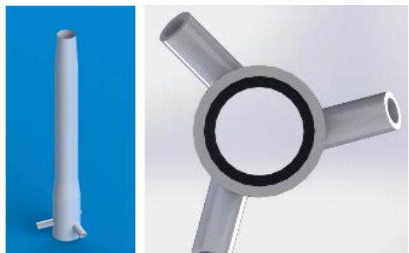
Fig. 2: Designed and rendered model of swirl nozzle and fluid element inside
