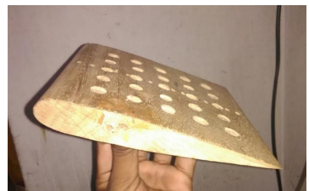
Figure 4: Constructed model with dimple surface
