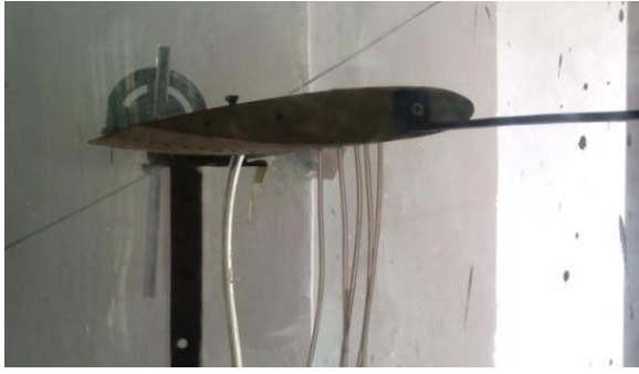
Fig 2: Experimental setup for measuring surface pressure on wind tunnel.
