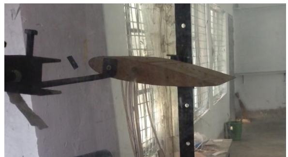
Fig 1: Experimental setup for measuring surface pressure on wind tunnel.
