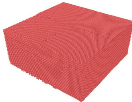
Fig. 1: An initial configuration of Co thin film with size of 20 \times 20 \times 10 nm.
