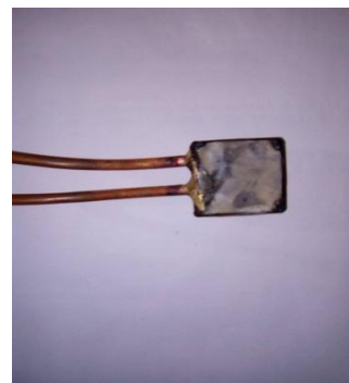
Fig 2: water block made of mild steel
