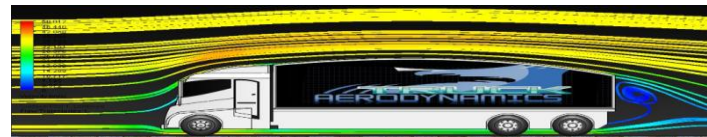
Fig. 17: Flow trajectories showing velocity flow over aerodynamic truck model
