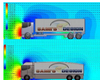
Figure 13: Pressure distribution over heavy duty truck and modified version of heavy duty truck
