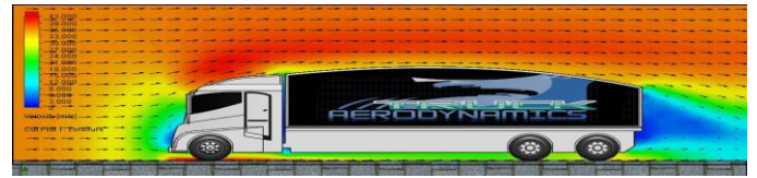
Fig. 11: Velocity distribution over modified aerodynamic truck model
