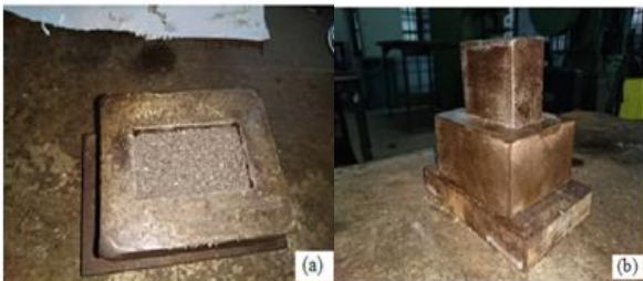
Fig. 1: (a) Brick samples in mould (b) Mould ready for pressing
