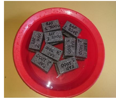
Fig. 4: Water curing of brick samples
