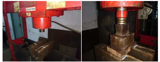
Fig. 2: (a) Hydraulic Press (b) Brick samples in the hydraulic press.
