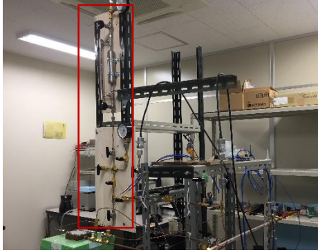
Fig.4: Connection between charging system (red rectangular) and LHP
