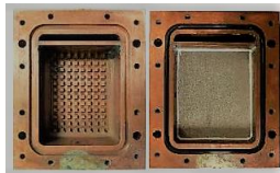
Fig.1: Evaporator with sintered stainless-steel wick
