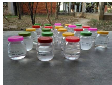
Figure 3: Samples kept in NaCl and NaOH solution containing bottles.
