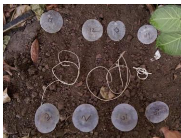
Figure 1: Sample being buried in Soil for Degradation Studies.
