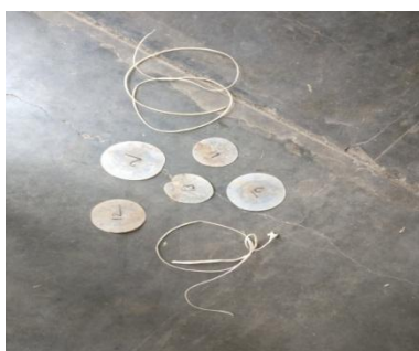
Figure 2: Samples taken out from soil for measuring weight and mechanical properties.
