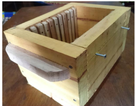
Fig. 2. A typical carrier to carry the test samples between the sample exposer and the laboratory during data collection.
