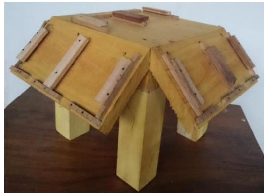
Fig. 1. A typical timber frame to expose the test samples at outdoor condition.
