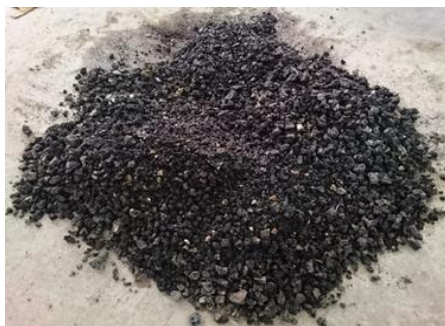
Fig. 1: Coarse slag sample in saturated surface dry (SSD) condition
