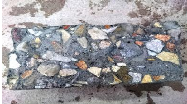
Fig. 8: Concrete specimen after splitting tensile strength test
