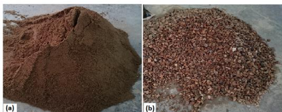
Fig. 2: (a) Fine aggregate (sand) sample in saturated surface dry (SSD) condition (b) Coarse aggregate (stone chips) sample in saturated surface dry (SSD) condition
