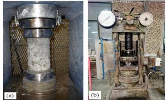
Fig. 6: (a) Compression test conducted on a concrete specimen with steel slag aggregates (b) Splitting tensile Test conducted on concrete specimen
