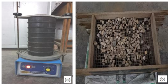
Fig. 4: Sieve analyses conducted to determine gradation
