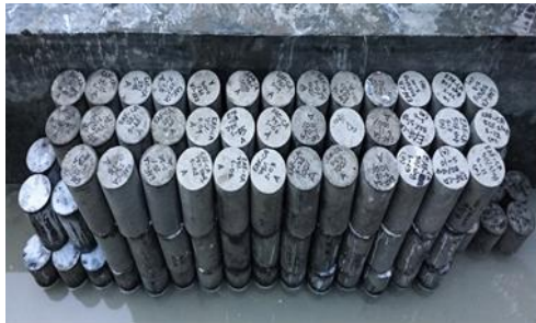
Fig. 3: Concrete cylindrical specimen after casting
