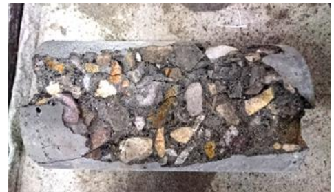
Fig. 7: Concrete specimen after compressive strength test
