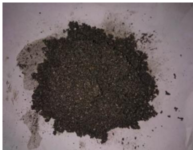
Fig. 1: Coarse slag sample in saturated surface dry (SSD) condition
