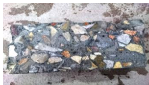
Fig. 8: Concrete specimen after splitting tensile strength test
