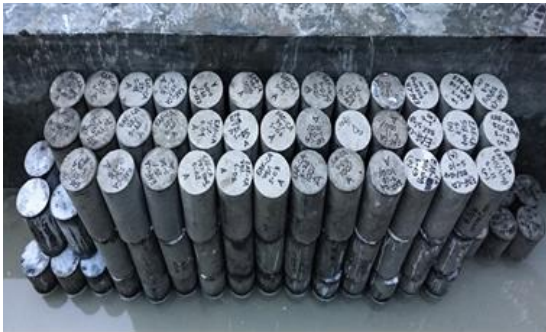
Fig. 3: Concrete cylindrical specimen after casting
