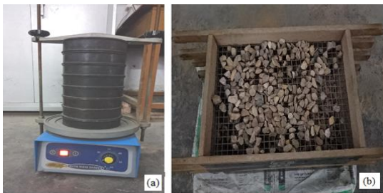
Fig. 4: (a) and (b) show sieve analyses conducted to determine gradation
