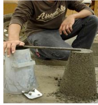
Fig. 5: Slump test being conducted on the concrete sample
