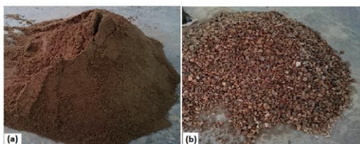
Fig. 2: (a) Fine aggregate (sand) sample in saturated surface dry (SSD) condition (b) Coarse aggregate (stone
