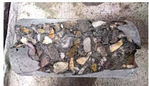
Fig. 7: Concrete specimen after compressive strength test
