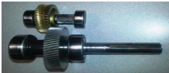
Fig. 3 Motor-shaft gear mechanism
