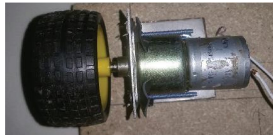
Fig. 1 DC Motor (12 V, 8.75 rpm)
