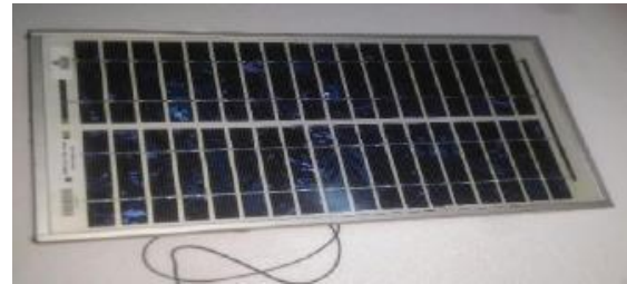
Fig. 4: Solar panel (Model: TBP 1210M, 17V, 0.6 A)
