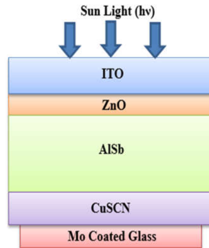
Fig.4: Structure of the AlSb Solar cell with Mo Coated Glass
