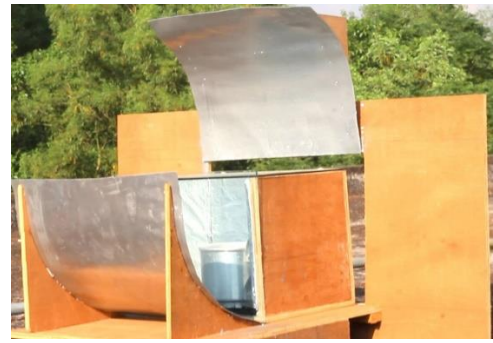
Fig. 7: Complete setup of the solar cooker.
