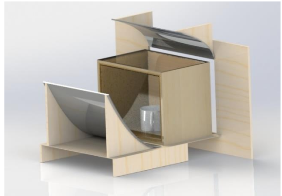
Fig. 1: Complete CAD model of wall integrated solar cooker.
