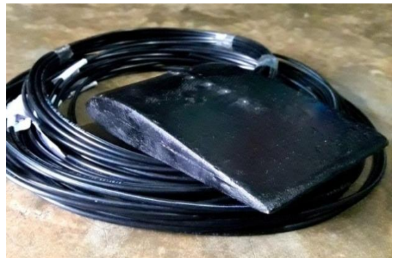
Fig.13: Airfoil models with chord length 14.5cm.
