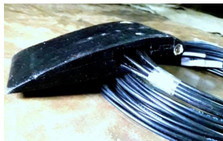
Fig.15: Airfoil model with chord length 16.5cm.
