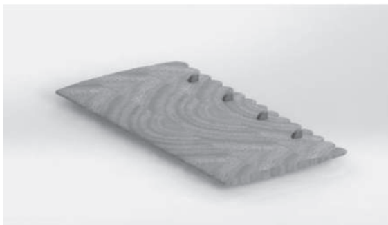
Fig. 5: NACA 0010 Airfoil with serrations and vortex generators
