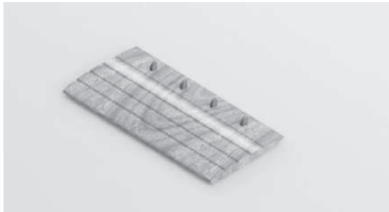
Fig. 5: NACA 0010 airfoil with strips and vortex generators
