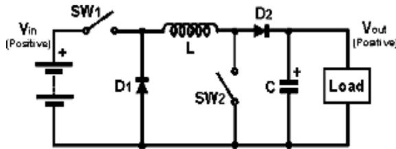
Fig. 6: Basic Buck-Boost converter
