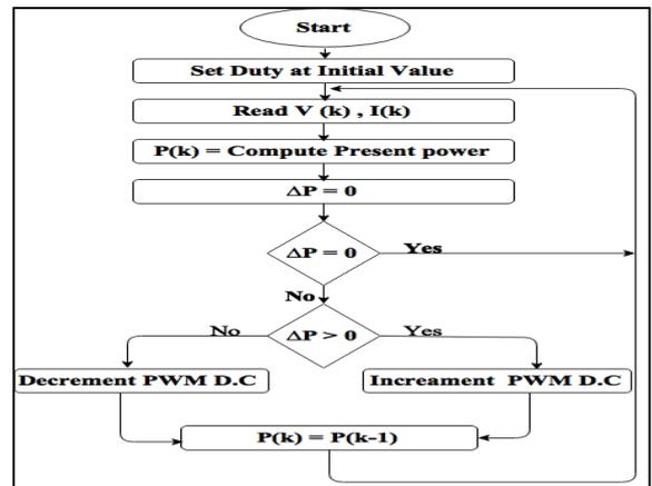
Fig.8: Flowchart of the Modified MPPT algorithm
