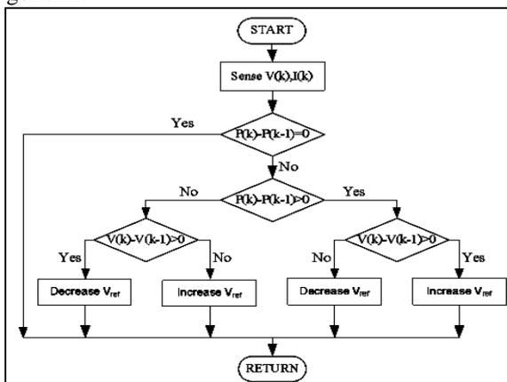
Fig.7: The flowchart of the P&O MPPT method
