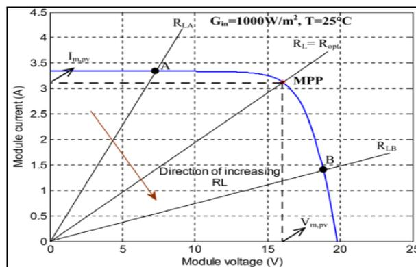
Fig.3: Solar Panel IV Curve with MPPT
