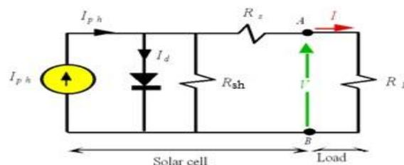
Fig.2: Equivalent Circuit of PV Solar Cell
