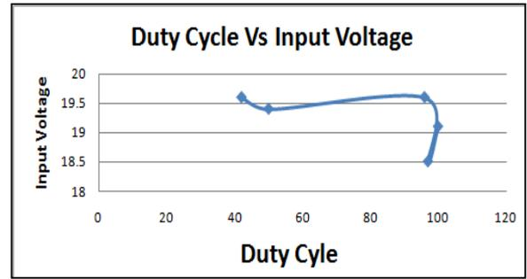
Fig.12: Duty cycle Vs. Input voltage characteristics
