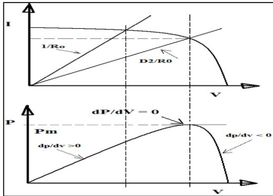
Fig.4: Working principal of any MPPT algorithm
