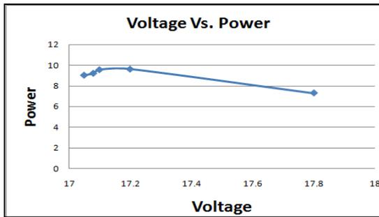
Fig.10: Voltage Vs. Power characteristics for Non-MPPT
